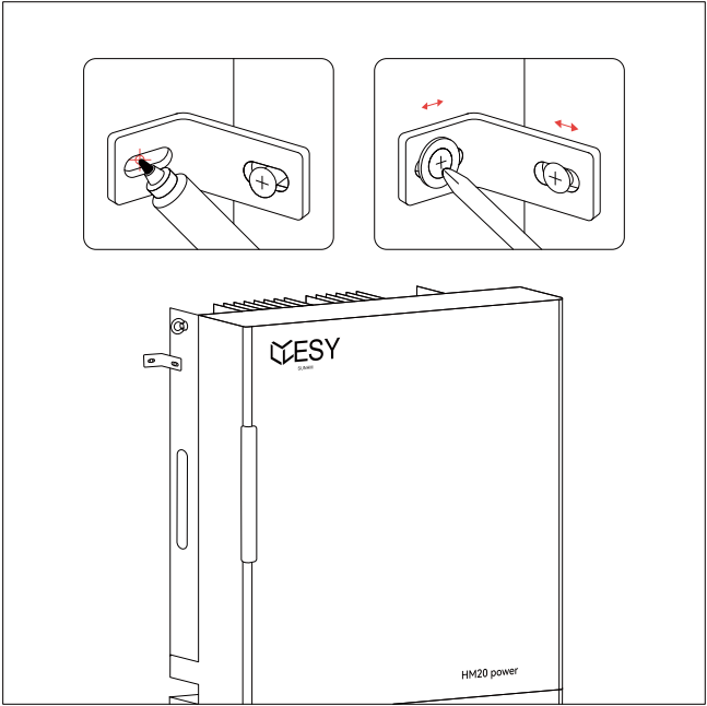
Step 6: Follow the same steps to install the inverter angle iron in the upper left corner of the inverter.
