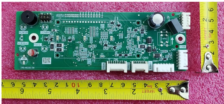
Figure 24. Top side view of LED board (optional)
